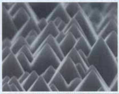
Wet etching Process
