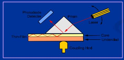
Make a narrow gab between the prism and the film using coupling (push) head
