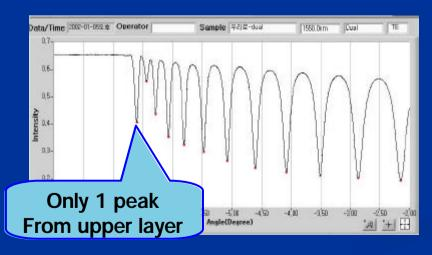
It is useful in the case that the difference of refractive index between upper and lower layer is small
